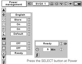
management to show this box. Choose one of three settings with the Point  $\blacktriangleleft$  buttons, and navigate to the timer with the Point  $\blacktriangle$  buttons and set time with the Point  $\blacktriangleleft$  buttons.
