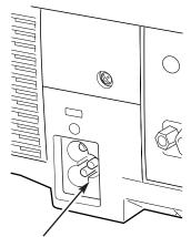
Connect the AC Power Cord (supplied) to the projector. The AC outlet must be near this equipment and must be easily accessible.
